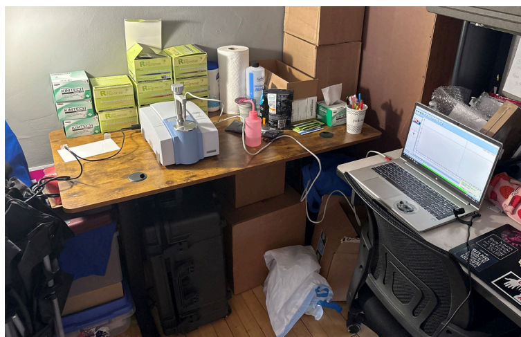
DCS station with FTIR machine, test strips, and results on laptop. (Photo provided anonymously.)
